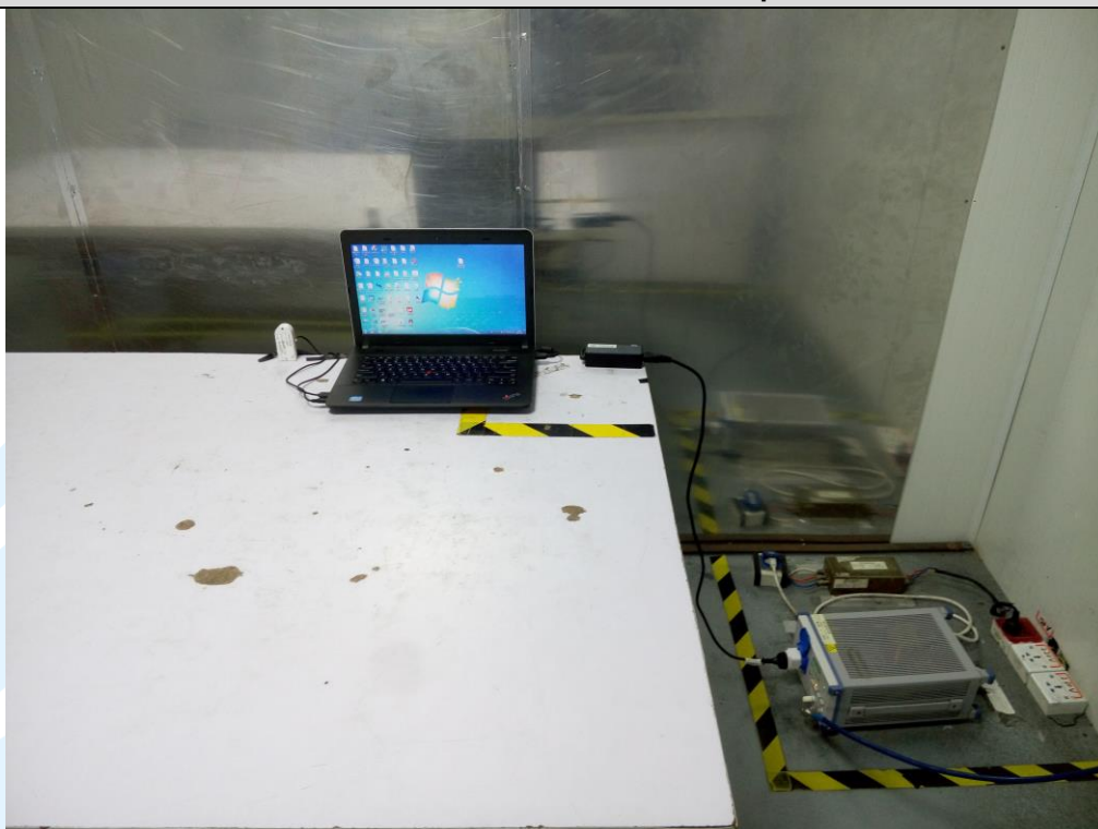
Conducted Emission Test Setup
