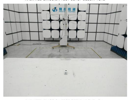
RADIATED EMISSION TEST SETUP ABOVE 1GHz
