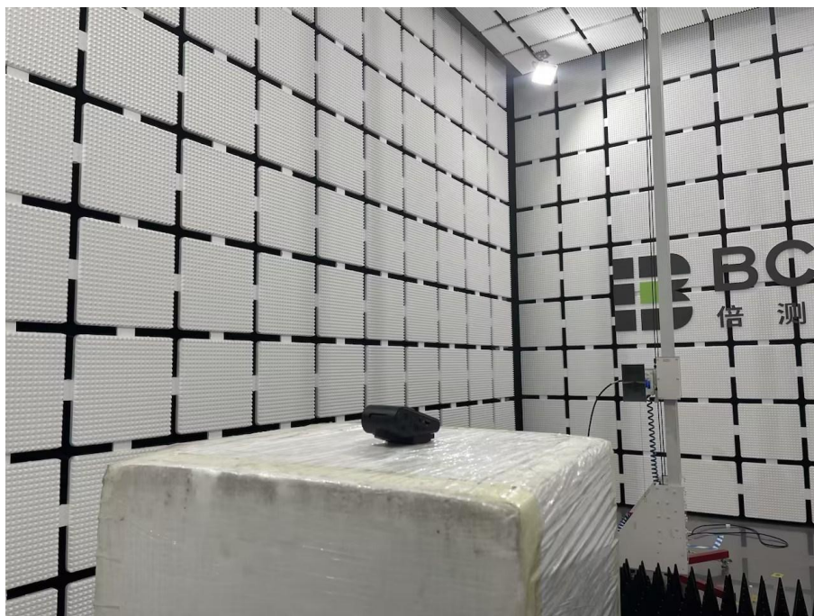
Spurious Emission Test Setup (Above 1GHz)
