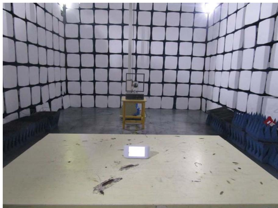
**Radiation Emission Test Setup (30MHz to 1GHz)**
