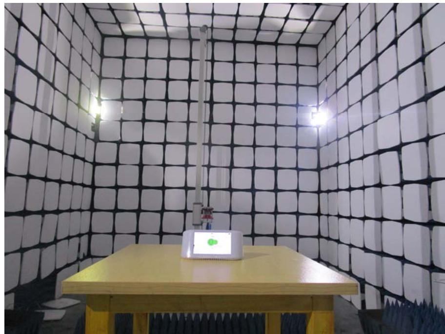
**Radiation Emission Test Setup (Above 18GHz)**
