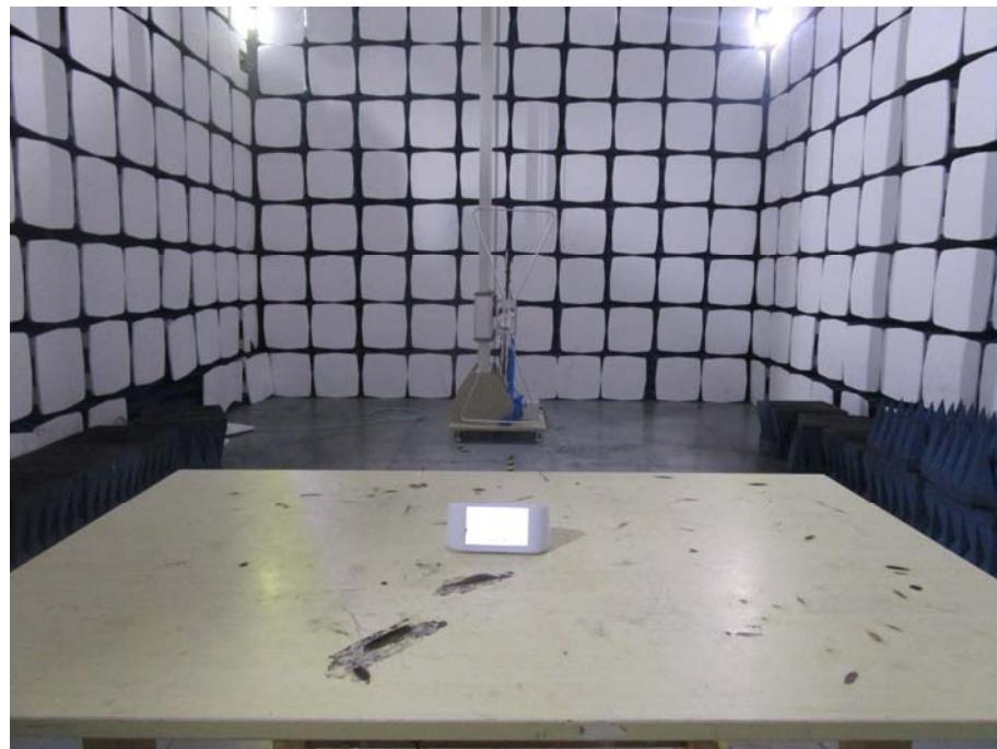
**Radiation Emission Test Setup (1GHz to 18GHz)**
