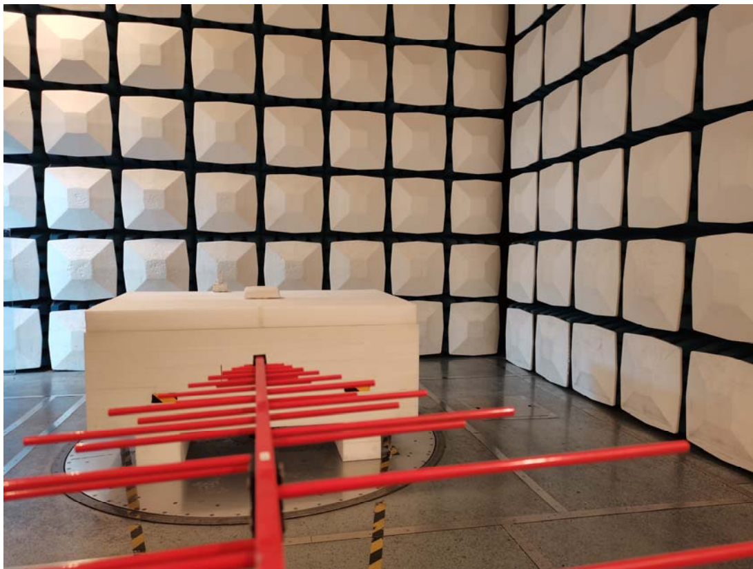
Radiated Emission Below 1GHz View-USB Adapter Mode
