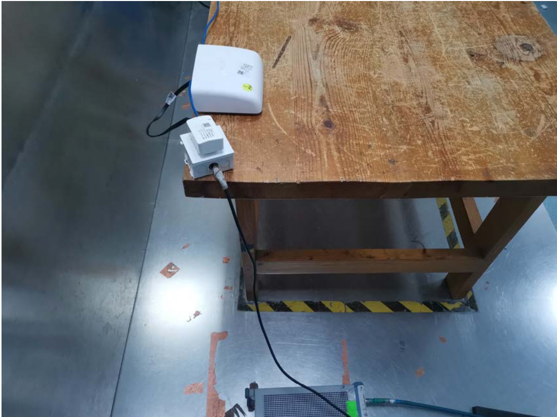
Conducted Emissions Side View-PoE Adapter Mode
