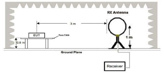
(2) Radiated Emission Test-Up Frequency 30MHz~1GHz
