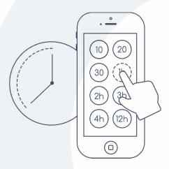
• iTraq Butterfly is NOT a real-time tracker. iTraq Butterfly operations are driven by a defined schedule. Using free iTraq Butterfly mobile application (iOS or Android), you can define the frequency of the location reports. These reports can range from every 15 minutes to every hour. The battery life depends on the frequency of the reports. The more reports per day – the shorter the battery life.
