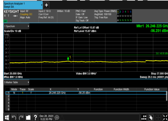
N48(20M)_DFT-s- OFDM BPSK Edge 1RB Left High CH
