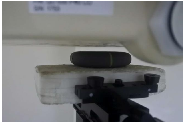
Back, Test Separation 5 mm
