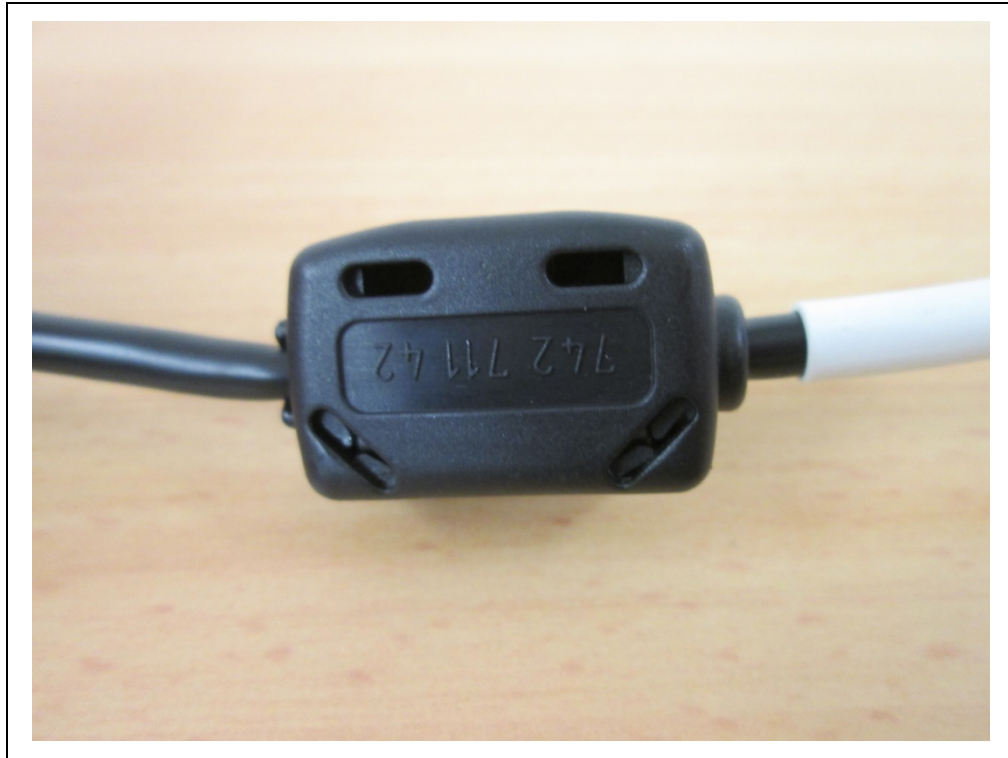
Photograph A4-3: Ferrit Würth 742 711 42 on charger cable
