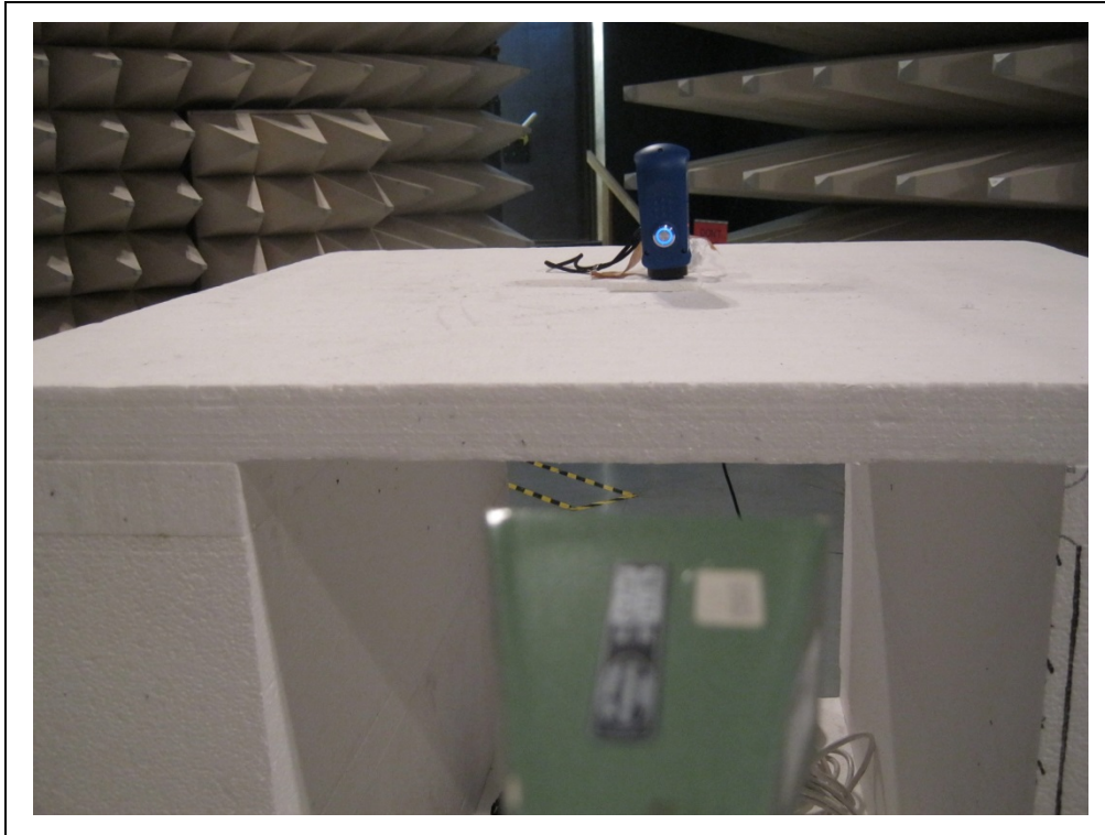
Photograph A1-7: Radiated emissions 18 – 26.5 GHz at 1 m distance
