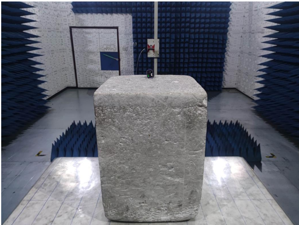
RADIATED EMISSION TEST SETUP ABOVE 1GHz
