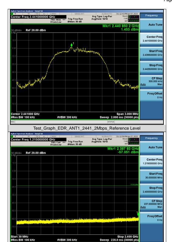
Test\_Graph\_EDR\_ANT1\_2441\_2Mbps\_Lower Band Emissions
