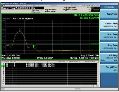
Note: The factor had been edited in the "Input Correction" of the Spectrum Analyzer. The GFSK modulation is the worst case and recorded in the report.
