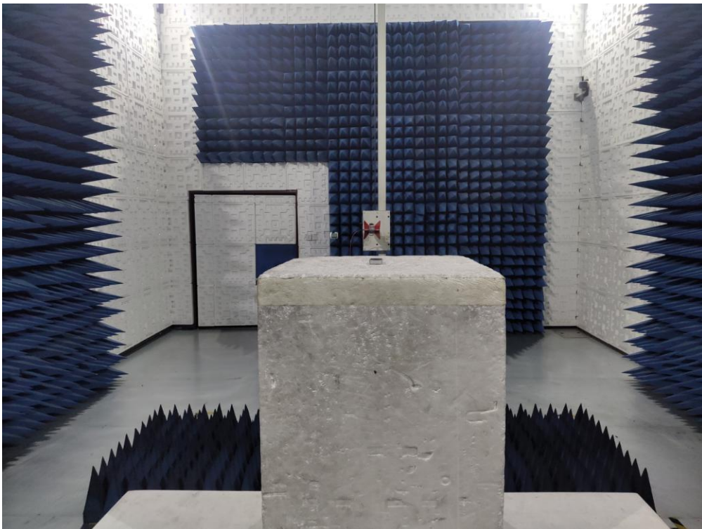
RADIATED EMISSION TEST SETUP ABOVE 1GHZ
