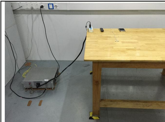
Conducted Emissions Test Setup Front View
