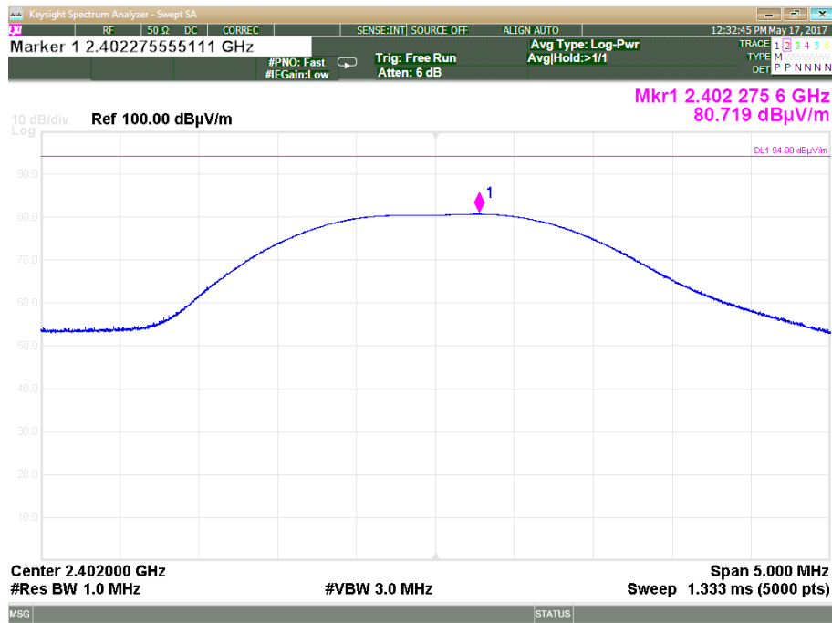
Plot 3.2.1: Radiated Emissions test, Vertical Polarization, Tx Modulated, Field strength of fundamental, Fc -2402
