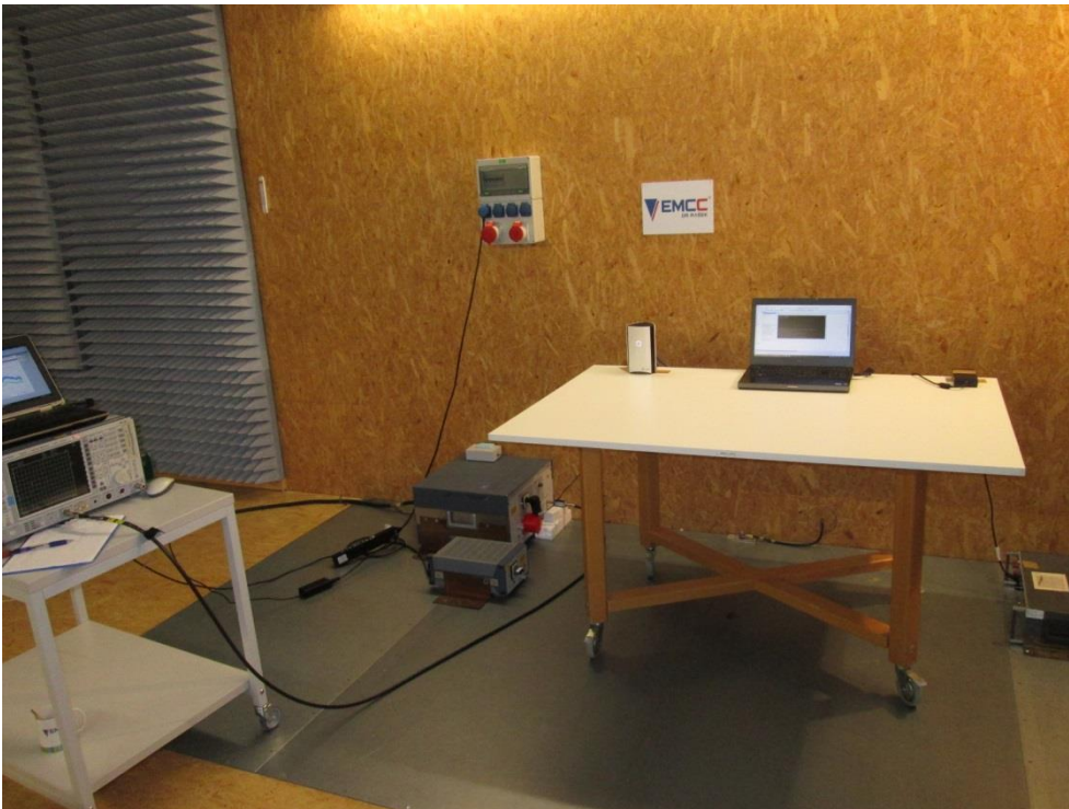
Photo A1-1: AC powerline conducted emissions measurement
