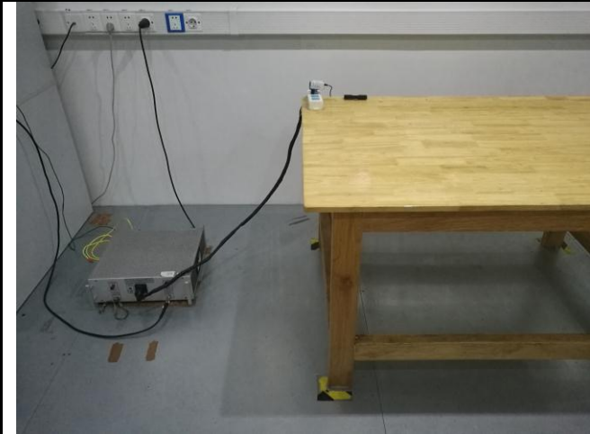
Conducted Emissions Test Setup Front View
