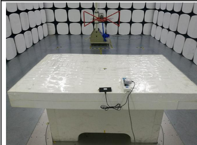
Conducted Emissions Test Setup Front View
