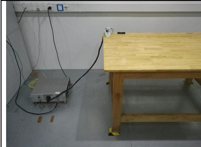
Conducted Emissions Test Setup Front View
