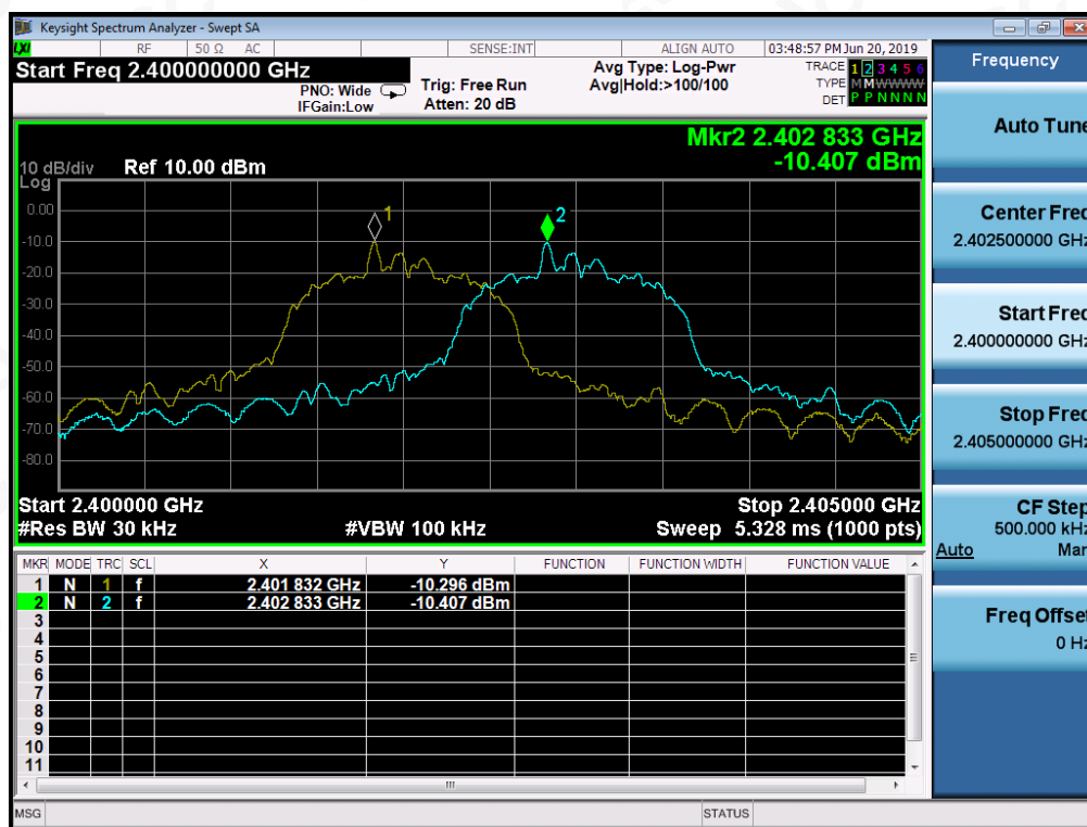
TEST PLOT FOR FREQUENCY SEPARATION
