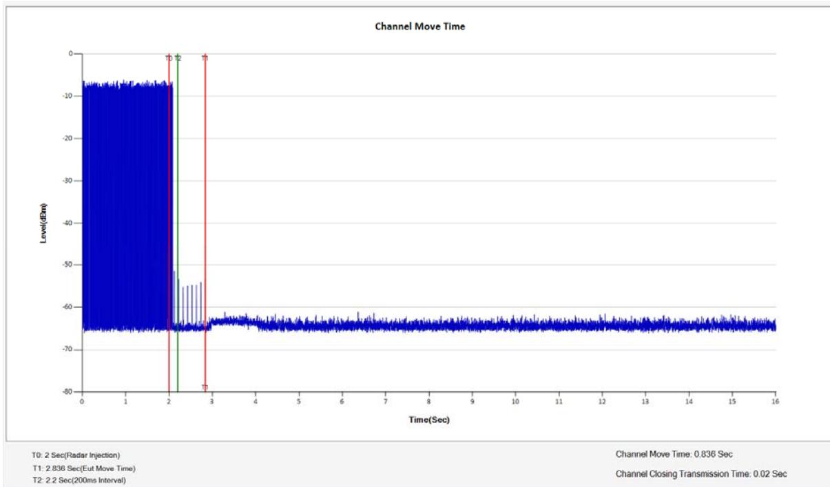
**Verdict:** Note: narrowing the sweep time as the good engineering process for the verification of transmission closing in 200ms
