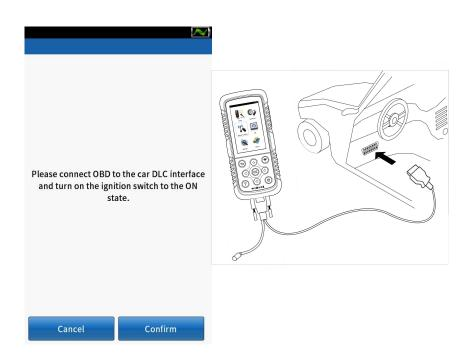
③ Click [Confirm], the device automatically read the sensor ID saved in the device board and display it on the screen.
