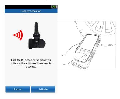
③ If the activation is successful, the OE sensor ID is displayed at the bottom of the screen.
