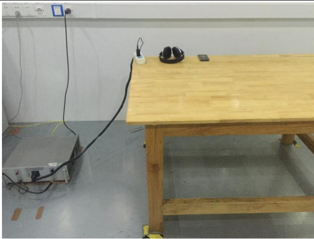
Conducted Emissions Test Setup Front View
