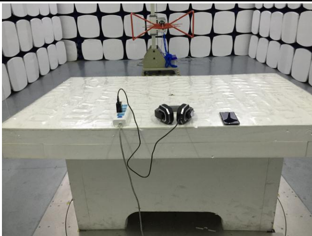
Conducted Emissions Test Setup Front View
