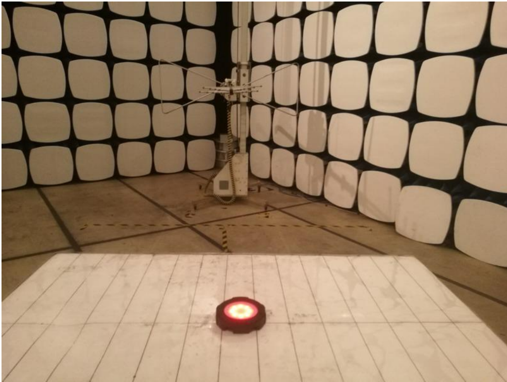
FCC RADIATED EMISSION TEST SETUP ABOVE 1GHZ
