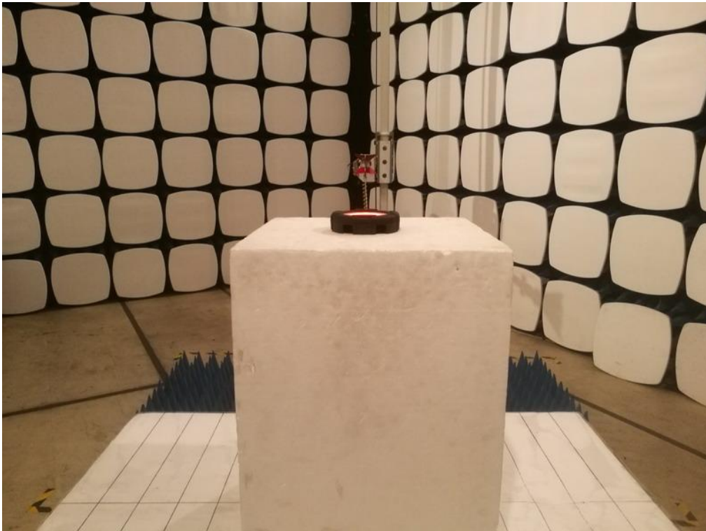
FCC RADIATED EMISSION TEST SETUP ABOVE 1GHZ
