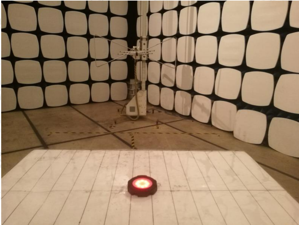
RADIATED EMISSION TEST SETUP ABOVE 1GHZ
