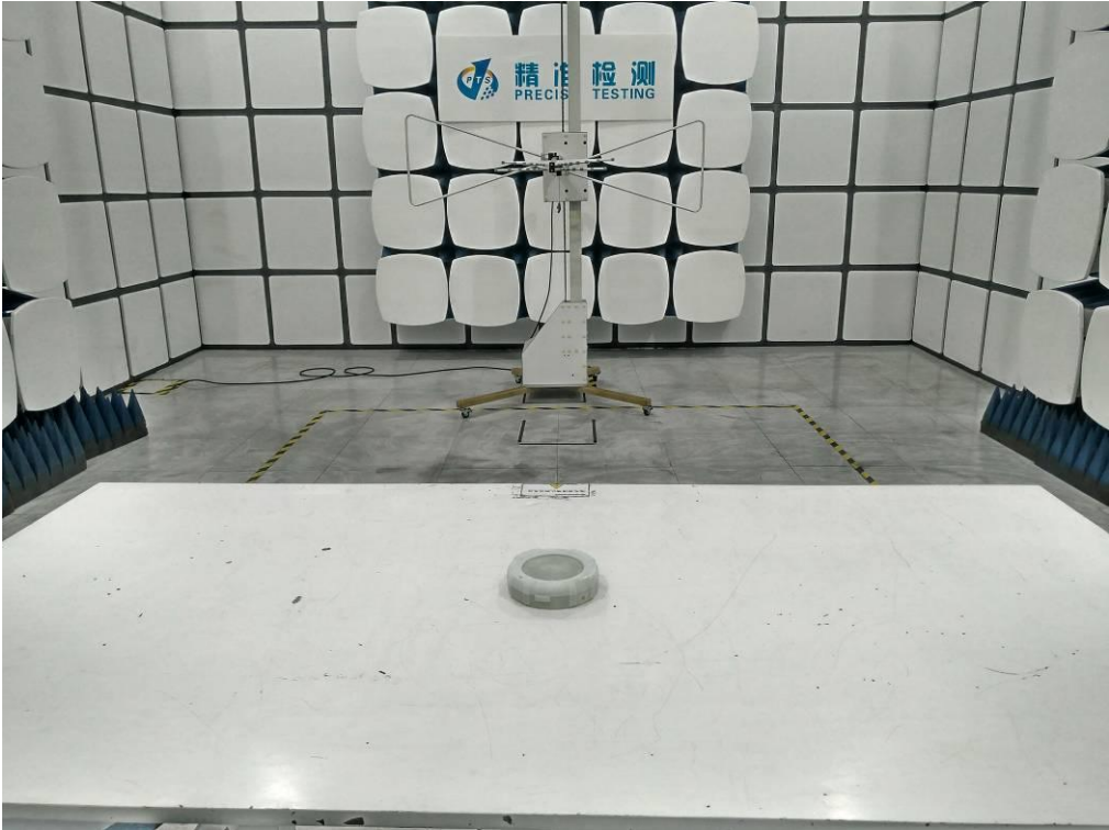
FCC RADIATED EMISSION TEST SETUP ABOVE 1GHZ
