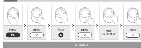
Preset lock time is 30 seconds. You can change lock time between 10-99 seconds.
