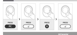
After you mount the lock on door, you need to set the door open direction. If you skip this step, lock doesn't work properly. Also please proceed this step when you reset the lock.
