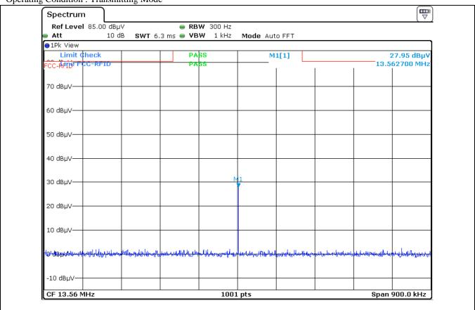
cc. to above test data, the field strength level of 13.562 7 MHz is 27.95 dBuV/m and the worst limit subject to 15.225 (b) and (c) is 80.5 dBuV/m, so the EUT meets the requirement.
