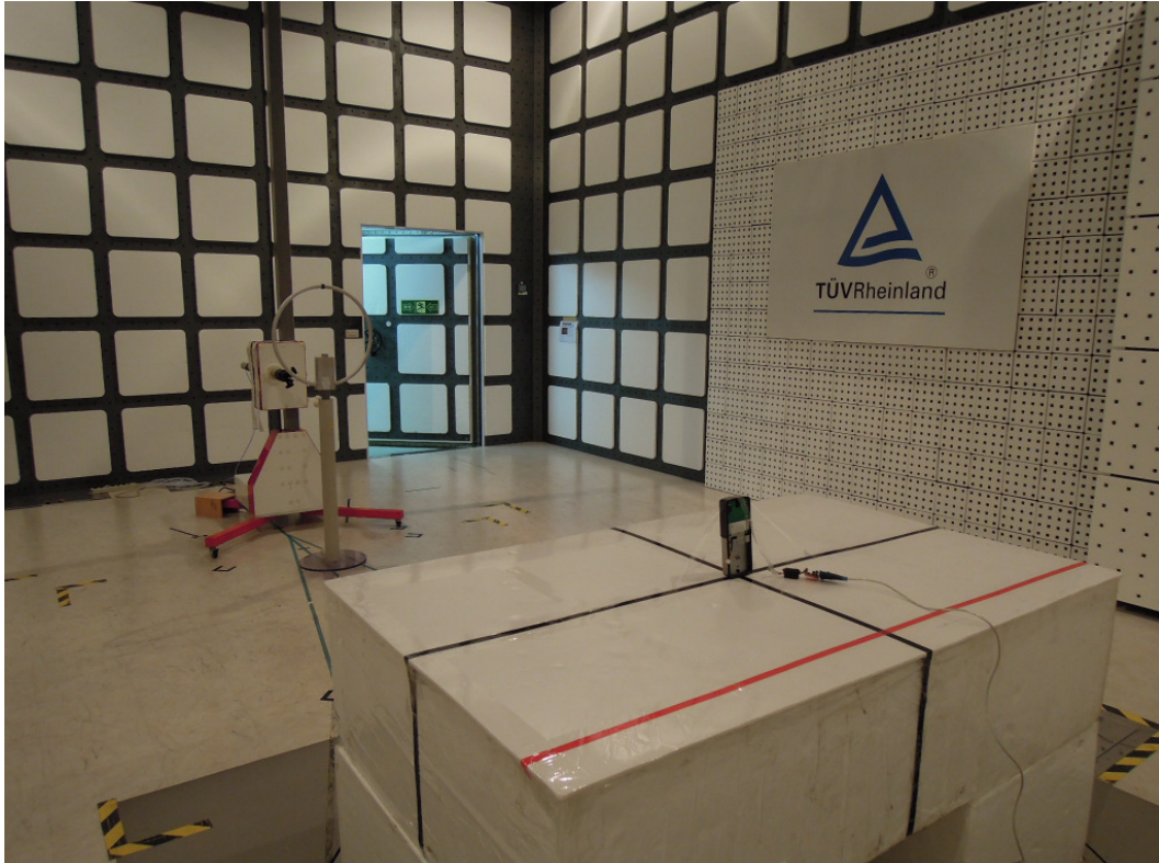
Photograph 3: Set-up for Spurious Emissions (Back View 2)
