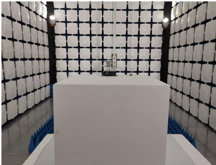
Above 1GHz for radiated emission test setup
