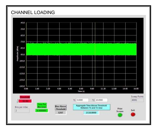
The level of traffic loading on the channel by the EUT is 21.18%
