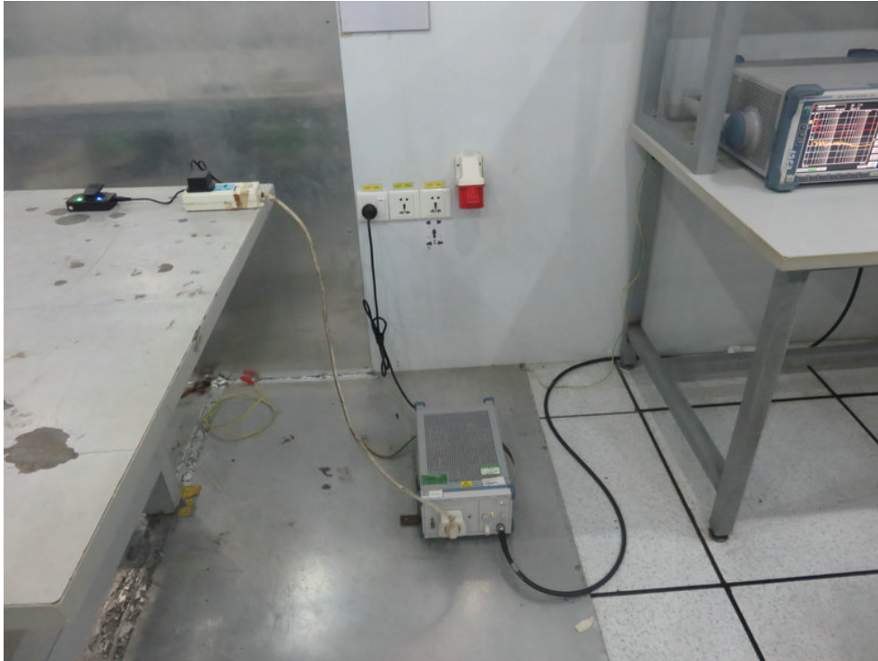
Photo of Conducted Emission Measurement
