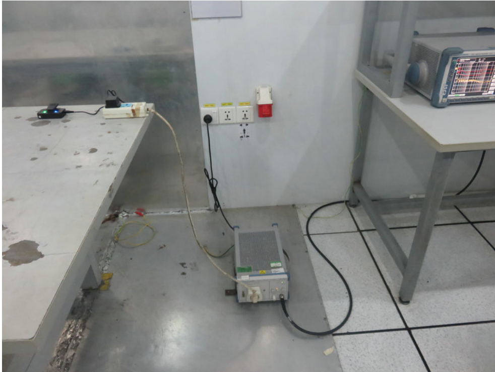
Photo of Conducted Emission Measurement
