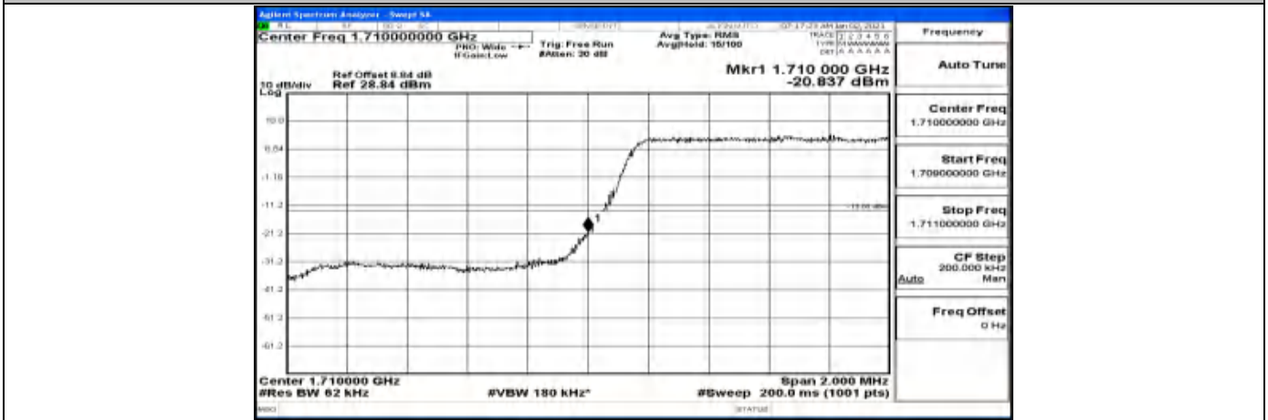
Band Edge Test Graph(s) (Channel Bandwidth: 1.4 MHz)_LCH_QPSK
