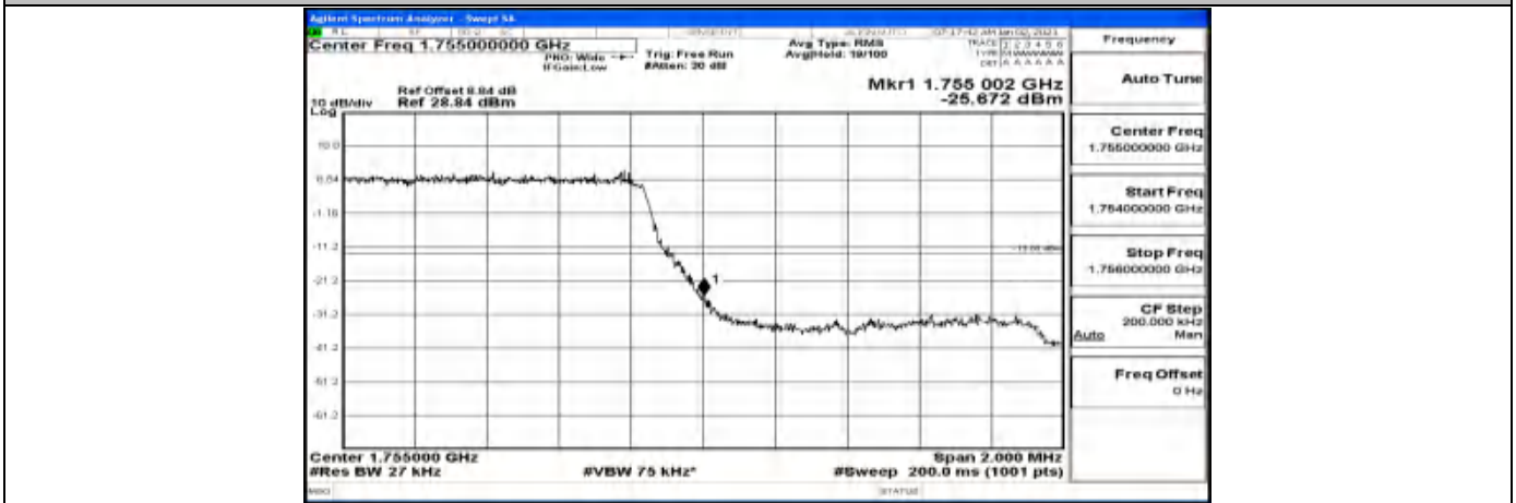
Band Edge Test Graph(s) (Channel Bandwidth: 1.4 MHz)_HCH_QPSK
