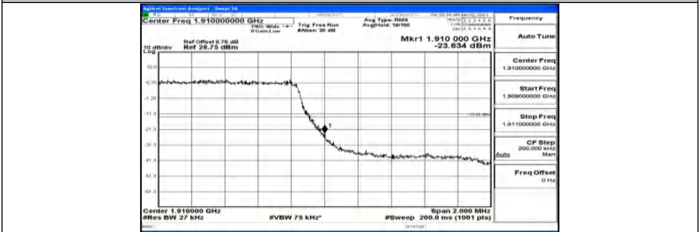
Band Edge Test Graph(s) (Channel Bandwidth: 1.4 MHz)_HCH_QPSK
