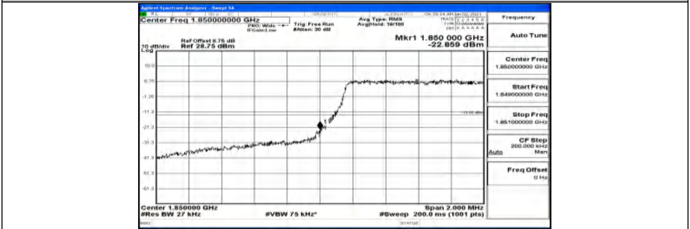
Band Edge Test Graph(s) (Channel Bandwidth: 1.4 MHz)_LCH_QPSK
