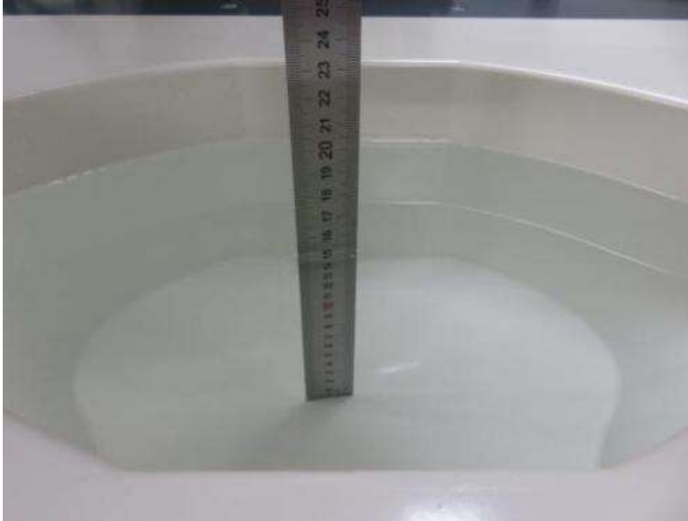
Photograph of the depth in the Body Phantom (2450MHz, 15.7cm depth)
