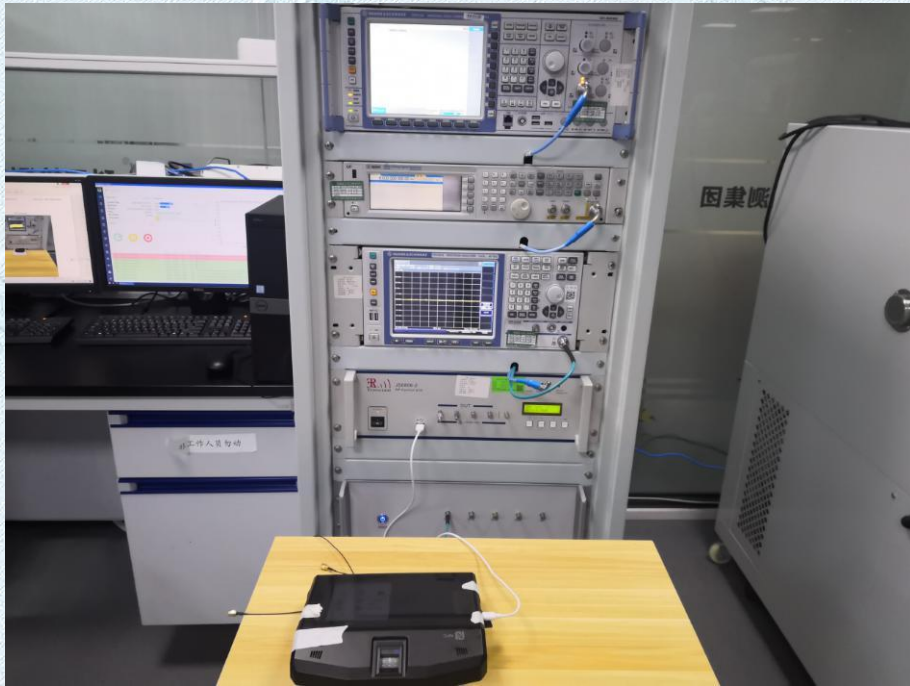
CONDUCTED EMISSION TEST SETUP
