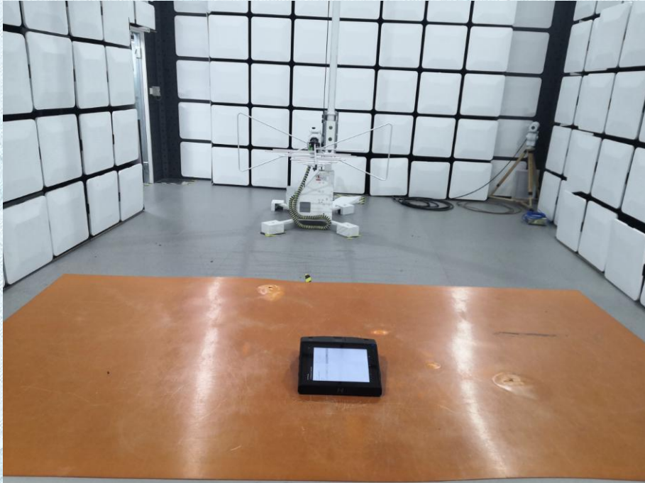
Radiated Measurement (Below 1GHz)
