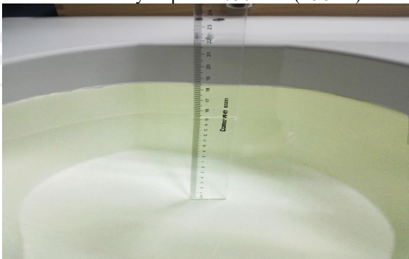
The Body Liquid of 1800MHz (15.2 cm)
