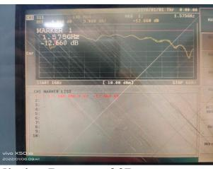
4-2.GPS Antenna Gain/Efficiency/Radiation Pattern of 3D 1575.000MHz
