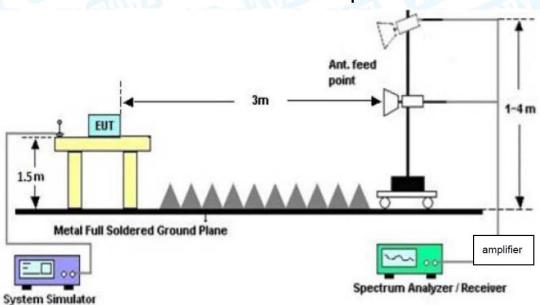
**Above 1GHz Test Setup**
