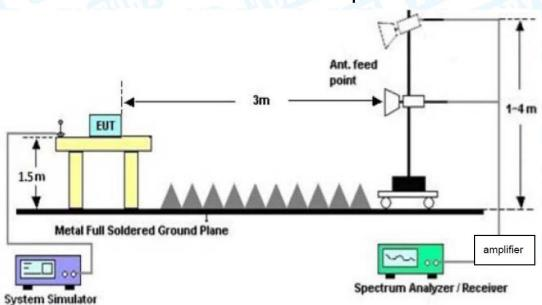
**Above 1GHz Test Setup**
