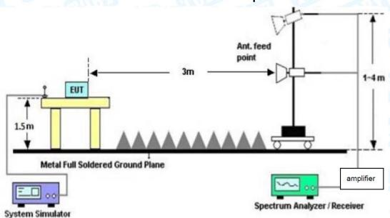
**Above 1GHz Test Setup**
