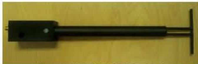
Figure 1 – MVG COMOSAR Validation Dipole
