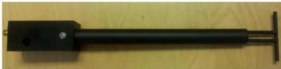
Figure 1 – MVG COMOSAR Validation Dipole
