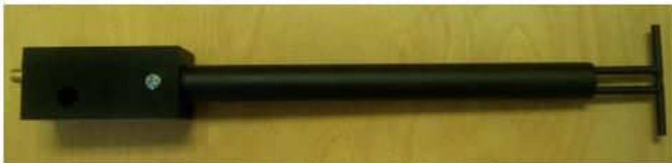
Figure 1 – MVG COMOSAR Validation Dipole
