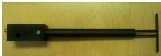
Figure 1 – MVG COMOSAR Validation Dipole
