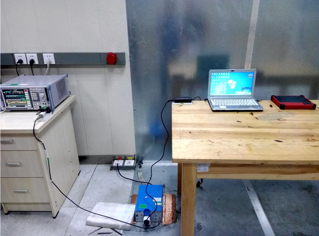
FCC RADIATED EMISSION TEST SETUP
