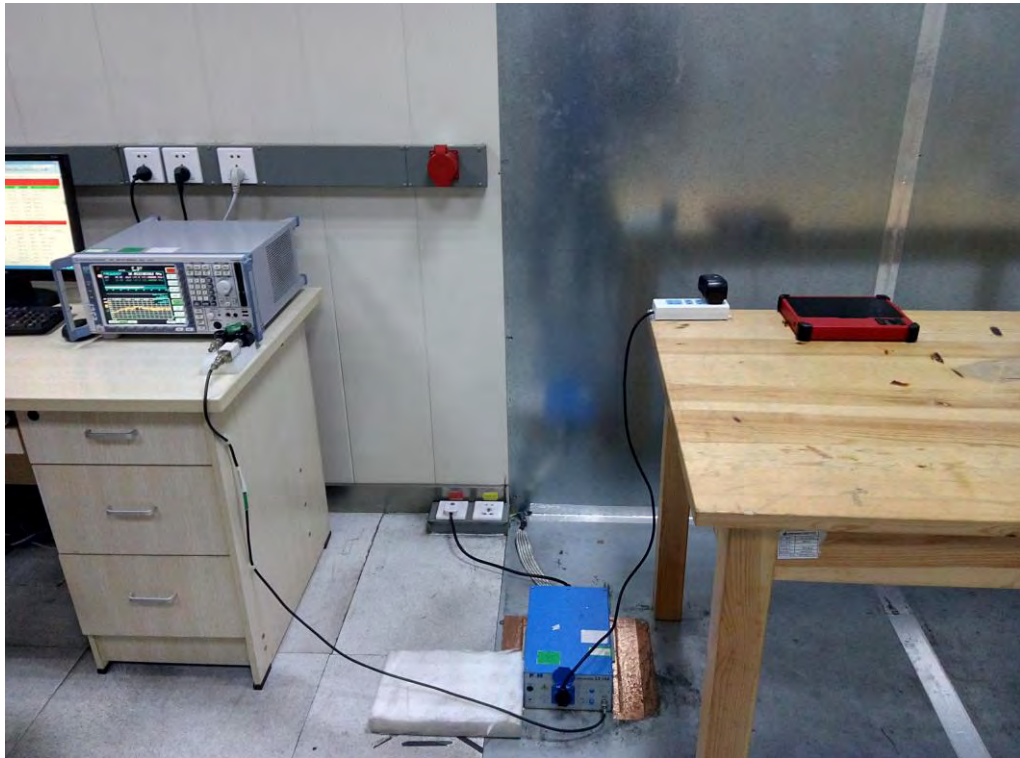
FCC RADIATED EMISSION TEST SETUP
