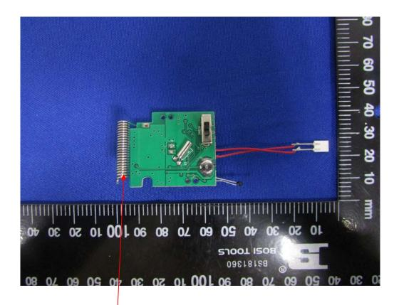
This is a internal helix antenna, antenna gain is -2dBi.
