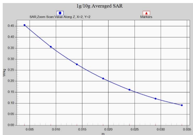
Fig.A.1- 12 Z-Scan at power reference point (CDMA BC0)
