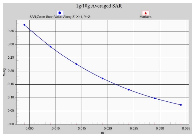
Fig.A.1- 30 Z-Scan at power reference point (LTE band26)
