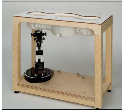
Picture C.10: SAM Twin Phantom
