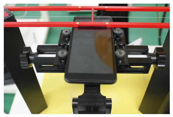
Picture 2: EUT Positioning for RF/T-coil
