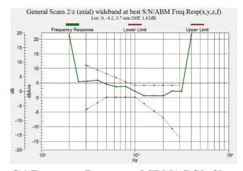
Figure C.1 Frequency Response of CDMA BC0\_Channel 384
