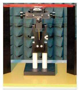
Figure 6.4 HAC Phantom & Device Holder
