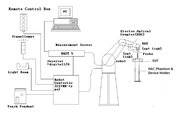
Figure 6.1 HAC Test Measurement Set-up
