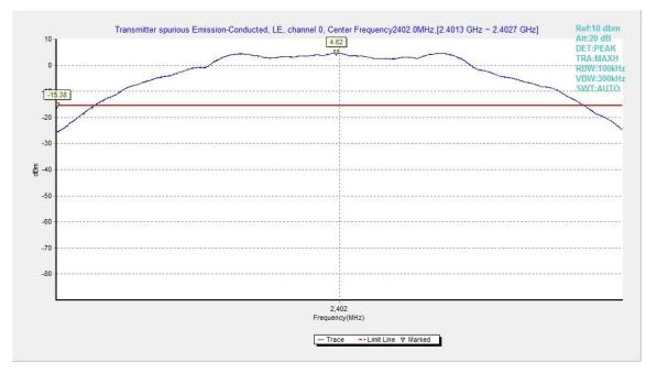
Fig.3. Transmitter Spurious Emission -Conducted: GFSK,2402MHz
