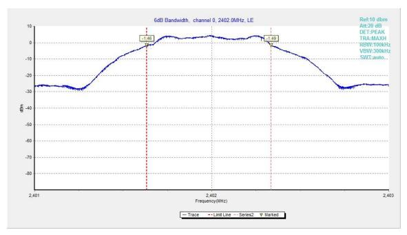
Fig.20. 6dB Bandwidth: GFSK, 2402 MHz
