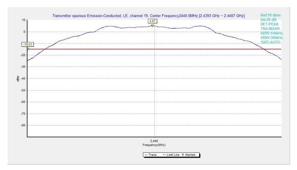
Fig.8. Transmitter Spurious Emission -Conducted: GFSK, 2440MHz
