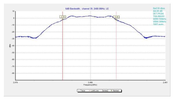
Fig.22. 6dB Bandwidth: GFSK, 2480 MHz
