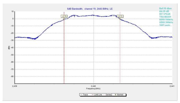
Fig.21. 6dB Bandwidth: GFSK, 2440 MHz
